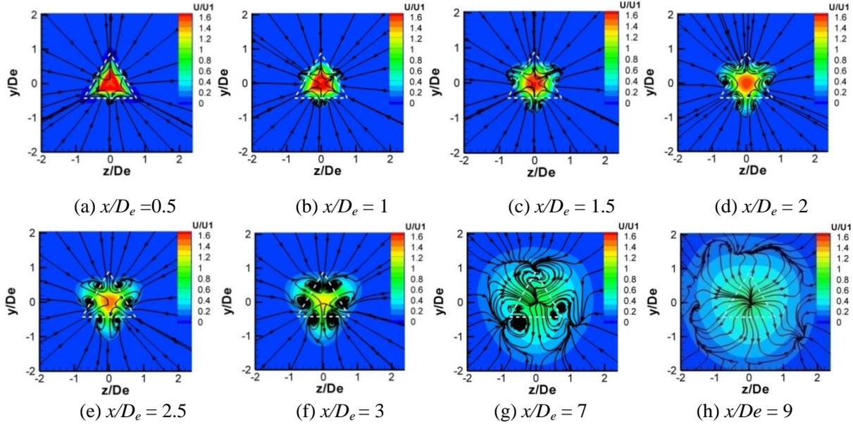
**Fig. 2** FTJ's cross-sectional views of longitudinal mean velocity contours and mean streamlines at different  $x/D_e$ .
