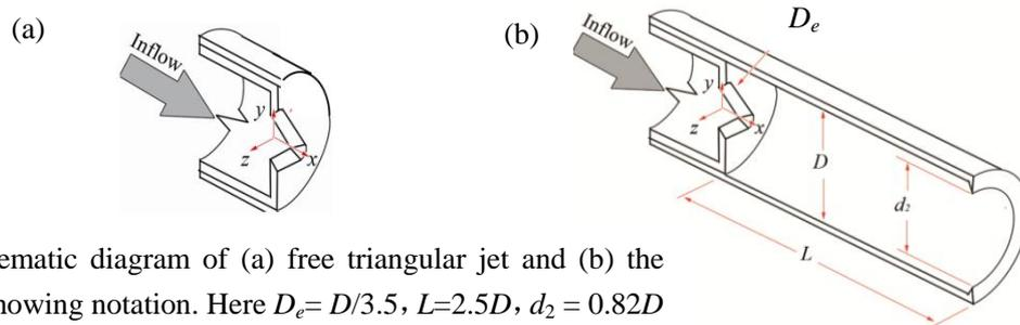
**Fig. 1** A schematic diagram of (a) free triangular jet and (b) the OTJ nozzle showing notation. Here  $D_e = D/3.5$ ,  $L = 2.5D$ ,  $d_2 = 0.82D$
