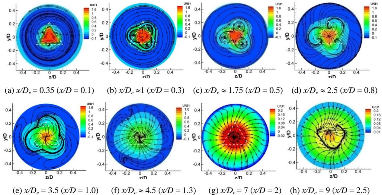
**Fig. 3** OTJ's cross-sectional views of longitudinal mean velocity contours and mean streamlines at different  $x/D_e$ .
